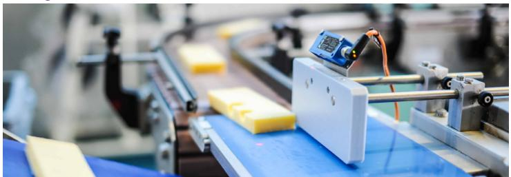
Proximity & position sensing (normally photoelectric) sense product flows and level controls (grains, powders & fluids) as well as temperature sensors. Plus other technologies such as barcode readers and vision sensors.
